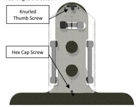
Use the Allen wrench to fix the Hex Cap Screw. Once the screw reaches its end position, no additional force may be applied.
