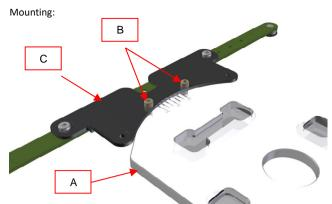
Screw the adapter plate onto the base plate using the M6x12 hex cap screws and Allen wrench 5 mm.
