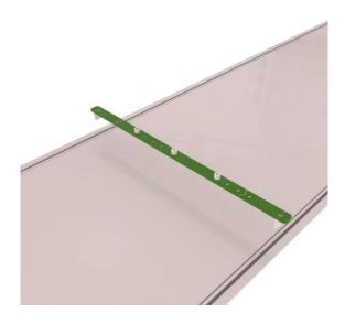
To position this 2-pin bar on such a couch, gently push the bar into the couch cut-outs. The bar itself should be flat on the surface of the couch. The 2-pin bar will be able to slide in a longitudinal direction. Always make sure that the bar is well positioned on the couch before indexing other hardware to the 2-pin bar.
