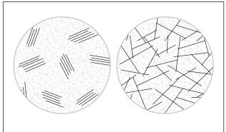
Shrinkage of nano composite material - schematic presentation of non-exfoliated (left) and fully exfoliated (right) nano clay composite material.
