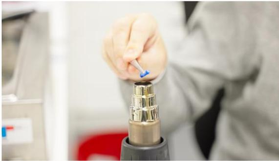
12. Cover the pegs on the inside of the Isoforce unit with the heated scrap material.
